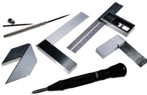
This set combines all the tools you need to have a starter set of marking tools. The set includes two solid steel engineer's squares (50 & 100mm), a 50mm centre square for marking the centre on round stock, an adjustable square fitted with a 150mm graduated rule, a scribe with spare tip and an adjustable centre punch. These are all housed in a plastic storage case.
