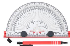
Inkra have reinvented the protractor by putting extra long guide slots at every 45 deg., 30 deg., 22.5 deg., 5 deg., 1 deg., and 0.5 deg interval to plot any angle with ease and absolute accuracy. If you take a few seconds to remove the T-bar you will also have an excellent 160mm rule with micro-fine marking holes at every millimetre.
