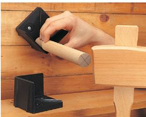
Made from aluminium, the Veritas Centre Finder uses a knife-edged steel blade to score the end of a workpiece. In soft wood the lines will be deep enough to hold the drive centre directly, so you won't need to make additional intersecting saw cuts in the drive end of your workpiece.
