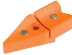
A useful companion tool for any tape measure, this odd-looking device helps you measure diagonals with confidence. An angled boss on the underside is designed to locate your tape securely on the inside or outside of corners while you take a measurement.
