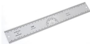
Find the exact centre of any work piece up to 300mm wide. In addition to top and bottom micro-fine marking holes at every 1/32" it also has a built-in protractor with guide slots at every 45 deg., 30 deg., 22.5 deg., and 5 deg. interval.
