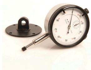
Graduated in 0.01mm with a range of 0 - 10mm. Fitted with rotating bezel with two moveable guides. Used to measure tolerances with machinery during setup. Supplied with a plastic storage case.
