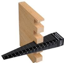
This aluminium gauge can be used in many ways, for setting fences, router bits and drill-press stops, as well as making any gap easy to measure and fill. The gauge is hard anodised, a process that makes the surface as hard to scratch as tool steel, yet leaves it easy to write on with a pencil. A simple, effective tool in metric graduations of 0.2mm. Features a fine tip .75mm
