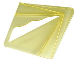
An out of balance piece of timber is more dangerous to work with, and requires more roughing down. Carbatec's Plastic Centre Find allows for very quick marking of the centre, simply place it on the end of the blank between the "V" wedge, and scribe the line, then rotate and repeat the process to get two crossed lines giving the centre point.
