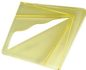
An out of balance piece of timber is more dangerous to work with, and requires more roughing down. Carbatec's Plastic Centre Find allows for very quick marking of the centre, simply place it on the end of the blank between the "V" wedge, and scribe the line, then rotate and repeat the process to get two crossed lines giving the centre point.
